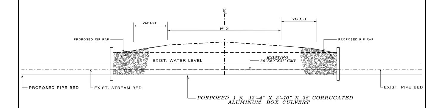
NOTES: \*PROPOSED 1 @ 13'-4" X 3'-10" X 36' CORRUGATED ALUMINUM BOX CULVERT TO BE BURIED 1.0' BELOW EXISTING STREAM BED
